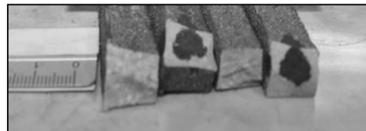
Fig. 3. A-F Hot cracking test for 0.17% Al addition to cast iron
