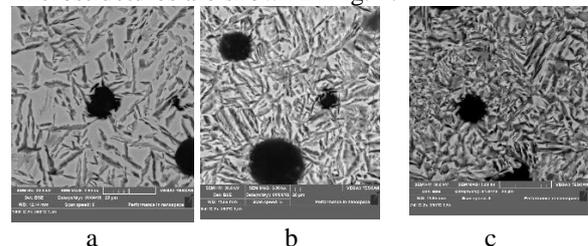
Fig. 1. Microstructure of cast iron austempered from the austenitizing temperature of: a) 1000°C, b) 850°C, c) 750°C
